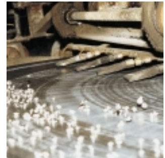
Blowing-off of the sprue from the permanent mould, illustration: Oetinger.
