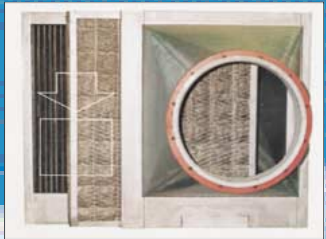
Horizontal gas flow: vane-type separator with agglomerator
