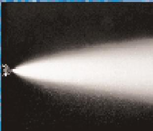
A primary prerequisite for gas conditioning is the capability to generate extremely fine droplets and to distribute these as evenly as possible in the gas flow. The nozzle lances employed for this purpose must be configured in accordance with the precise requirements of the plant concerned.
